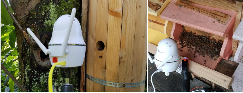
Figure 1: Non-invasive camera setup to record the bee videos.
